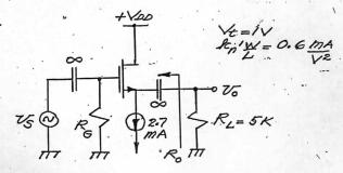
a) For the circuit shown, determine the value of  $g_m$  and draw the small-signal equivalent circuit using the "T" model for the MOSFET. (Label all model and circuit elements)
