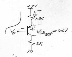
For the given values of  $V_B$  below, estimate  $I_B$ ,  $I_E$ ,  $I_C$  and the collector voltage,  $V_C$ , assuming  $\beta$  very large,  $|V_{BE}|=0.6V$  and  $|V_{CE(sat)}|=0.2V$ .
